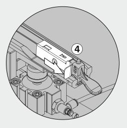
3 - Open the slider closing trigger.
