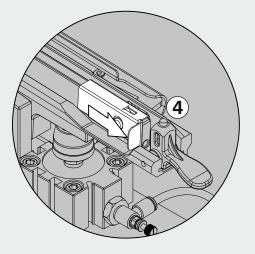
3 - Open the slider closing trigger.
