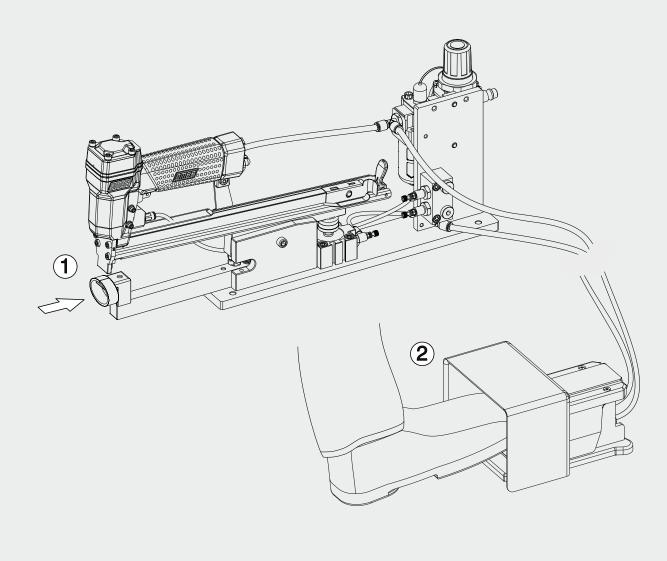
A front side opening adjustment must be carried out to allow an easy insertion of the material to be fastened.
