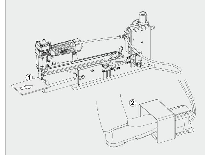
A front side opening adjustment must be carried out to allow an easy insertion of the material to be fastened.
