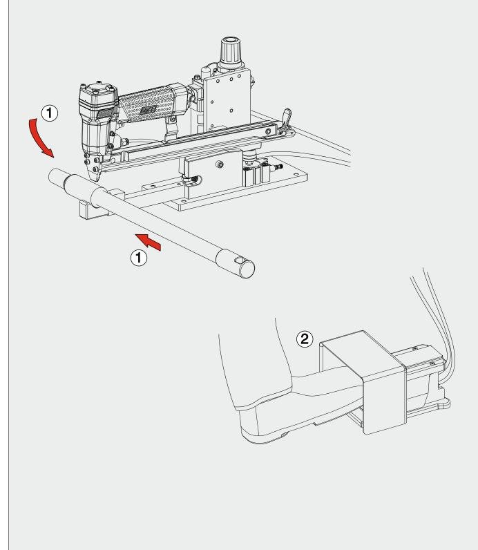
A front side opening adjustment must be carried out to allow an easy insertion of the material to be fastened.
