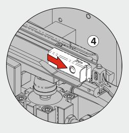
3 - Open the slider closing trigger.
