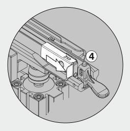
3 - Open the slider closing trigger.
