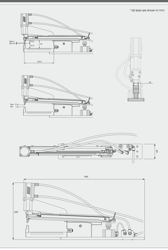
A front side opening adjustment must be carried out to allow an easy insertion of the material to be fastened.
