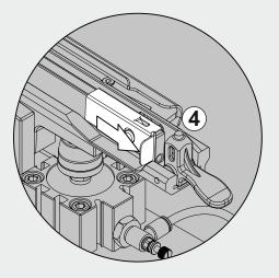
3 - Open the slider closing trigger.
