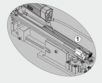
1 - Pull the pusher backwards and lock it at the stop position at the rear of the tool, this will open the movable hold down
