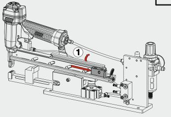
1 - Pull the pusher backwards and lock it at the stop position at the rear of the tool, this will open the movable hold down
