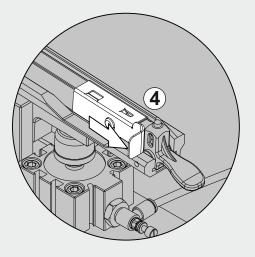
3 - Open the slider closing trigger.
