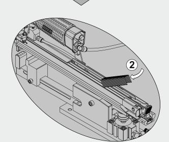
1 - Pull the pusher backwards and lock it at the stop position at the rear of the tool, this will open the movable hold down
